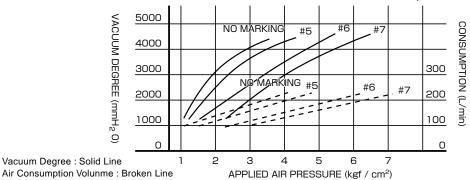
2) Max. Discharge Pressure and Air Consumption Volume (In the case of DISCHARGE)
